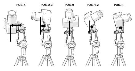
6.2. Pointing East. When the weight of the camera setup tends to rotate the ball-head in an anticlockwise direction, the spring should be tensioned to one of the numbered teeth, based on how strong the imbalance is. By tensioning the spring in position 5 (worst case scenario) a weight of up to 2kg can be balanced – i.e. pointing to the Zenith with the camera body towards the east in respect to the ball-head.
