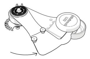
**7.7.** Push the assembled arm back to it's original position. Make sure to keep the winding knob remains "up-side down".
