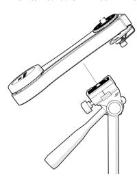
**4.1.** The MiniTrack LX2 NS is compatible with any  $\frac{1}{2}$ " tripod plate (#9 Side B). Set the mount to the tripod's plate (not supplied) as shown. Make sure that the mounts set so the inclination can be adjusted.
