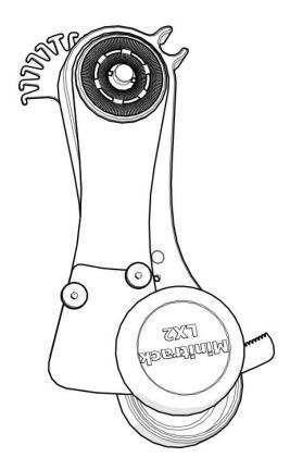
The south hemisphere configuration is to be used below the equator. In the southern hemisphere, the sky "rotates" on the opposite direction, i.e. from West to East. For that reason, it is necessary to add an additional arm (D) to the mount and invert the sense of the timer's movement.
