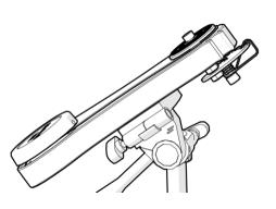
**4.2.** Make sure the mount is parallel to the adapter base. This is important because the inclination needs to be fine-tuned to set the mount in station.
