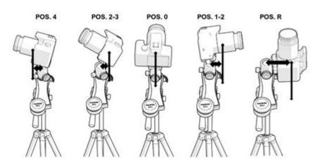
9.2. Pointing West. When the weight of the camera setup tends to rotate the ball-head in a clockwise direction, the spring should be tensioned to one of the numbered teeth, based on how strong the imbalance is. By tensioning the spring in position 5 (worst case scenario) a weight of up to 2kg can be balanced – i.e. pointing to the Zenith with the camera body towards the west in respect to the ball-head.
