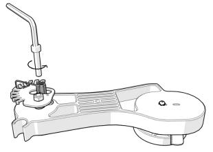
**8.1.** Release and Remove the post using an 4mm Allenkey (not included).
