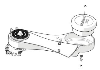
**7.4.** Remove the winding knob (#6 Side A) and the timer screw and washer (#12 Side B) as shown.
