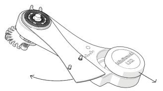
**7.3.** Push the winding knob (#6 Side A) away from the arm (#4 Side A) in order slide the arm to the left – please push it slightly only and make sure the spring (#10 Side B) is not impeding this movement.
