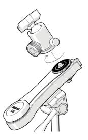
**4.3.** We recomend using a ball-head to operate the MiniTrack LX2 NS. It already has a pre-installed 3/8" thread adapter (factory assembled). If you already have a 3/8" ball-head and wish to use it just thread it to the adapter (#2 Side A). You can also use ¼"-20 ball-heads. For that you need to remove the pre-installed 3/8" ball-head adapter and replace it by the ¼"-20 adapter (C). Use the supplied adapter key (A).
