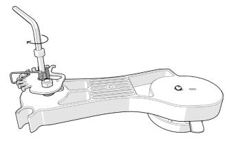
**8.2.** Move and align the Spring to the adjacent position. Insert the Spring post and re-tighten it with the Allenkey (not included). Exert caution, do not overtighten it.
