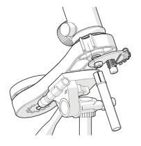
**10.2.** To align the mount to the SCP with more precision slide the polar finder (B) to the polar finder holder (1 Side A).
