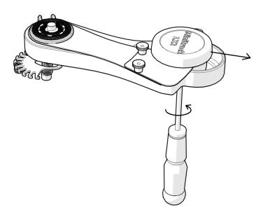
**7.8.** Push the arm to the timer and the winding knob against the teeth. Use a Philips-style screwdriver (not supplied) to fix it in place. It is important to not overtighten the screw as it may damage the timer and its performance.
