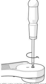
**7.2.** Release and unscrew the timer screw with washer (#12 Side B) using a Philips-style screwdriver (not included).
