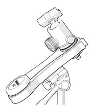
**4.4.** The ball-head must be securely fixed. Make sure to tighten it well. All the weight from the camera will rest on the ball-head. Besides that, a well-fixed ball-head ensures that there will be no slippage during long-exposures. At this point, it is important that the ball-head knobs are also tight. This prevents movement when installing the camera.
