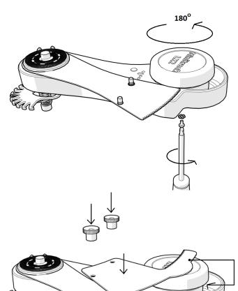
**7.5.** Turn the winding knob (#6 Side A) 180 degrees form it's original position(up-side down) and screw back the timer screw and washer (#12 Side B) but **do not tighten it yet!**
